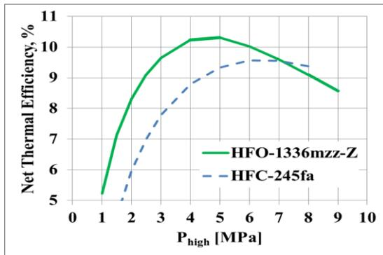
Figure 4: Net thermal efficiency (in %) of ORCs with HFO-1336mzz-Z as the working fluid compared to HFC-245fa (no recuperator;  $T_{exp,in}=225$  °C;  $T_{cond}=75$  °C;  $\Delta T_{subc}=5$  K;  $\eta_{EXP}=0.75$ ;  $\eta_{PUMP}=0.50$ ).
