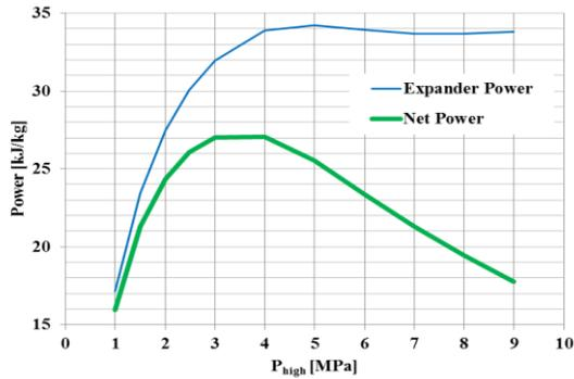
Figure 3: Expander and net power per kg from ORCs with HFO-1336mzz-Z as the working fluid (no recuperator;  $T_{exp,in}=225$  °C;  $T_{cond}=75$  °C;  $\Delta T_{subc}=5$  K;  $\eta_{EXP}=0.75$ ;  $\eta_{PUMP}=0.50$ ).
