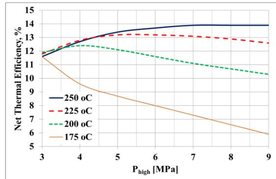
Figure 5: Net thermal efficiency (in %) of transcritical Rankine cycles with HFO-1336mzz-Z as the working fluid (no recuperator;  $T_{exp,in}=175-250$  °C;  $T_{cond}=75$  °C;  $\Delta T_{subc}=0$  K;  $\eta_{EXP}=0.85$ ;  $\eta_{PUMP}=0.65$ ).
