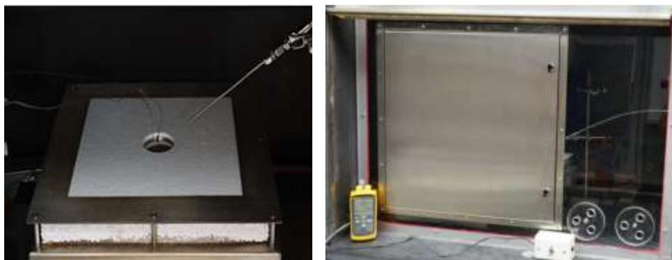
**Figure 1** The picture on the left shows the ceramic hot plate with the attached planchet. The refrigerant spray line can also be seen. The picture on the right shows the complete enclosure which is contained within the fume hood. It should be noted that before turning on the hot plate, the enclosure varied in temperature between 18-20 °C (64.4- 68 °F ) and was draft-free as measured by an anemometer.
