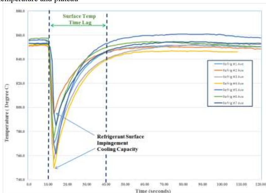
**Figure 2** HSI Profile vs Time for 2L Refrigerants tested at 850°C.
