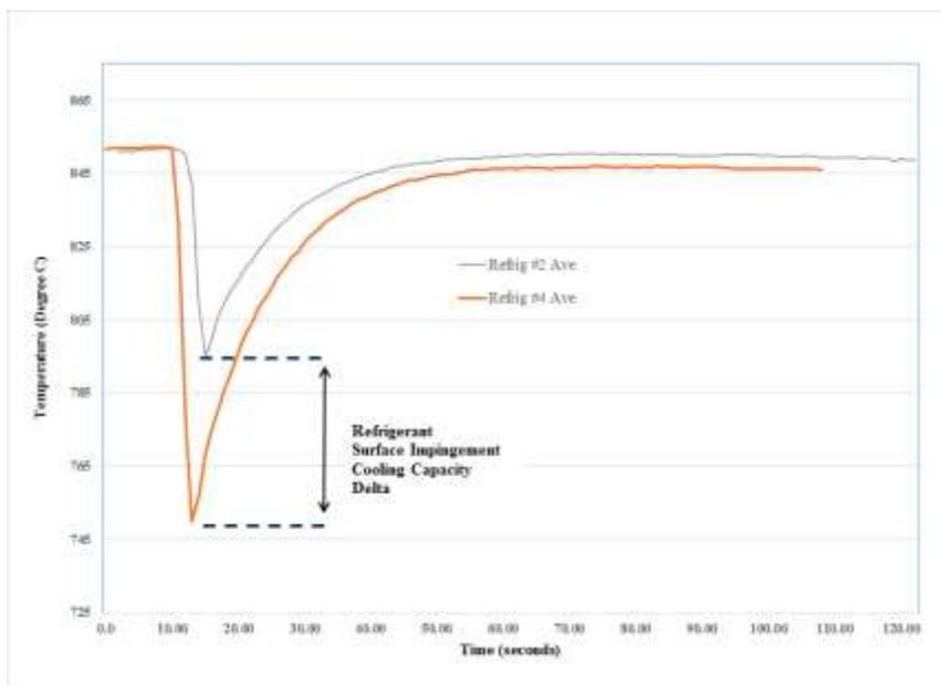
**Figure 3** HSI Profile vs Time for Refrigerant #2 and Refrigerant #4 tested at 850°C.
