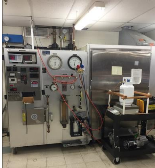
Figure 2. Compressor calorimeter used to experimentally test R-449A versus R-22
