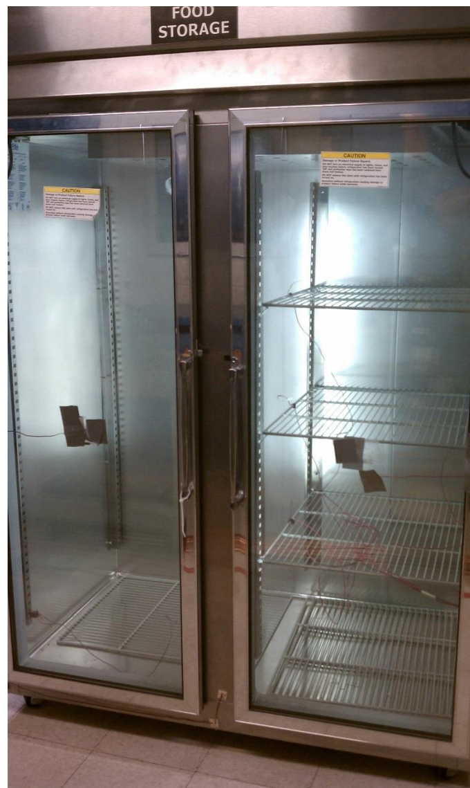
Figure 1: R-404A Reach-in freezer used in experimental testing
